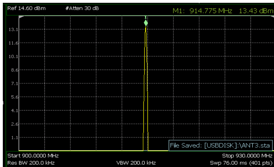
Figure 6.6 Antenna power reception. Power levels were monitored and recorded using a portable spectrum analyzer. When aligned with the RF field, and located at a distance of 15cm from the transmitter, the antenna receives 13.43dBm (22mW) of power at a center frequency of 915MHz.
